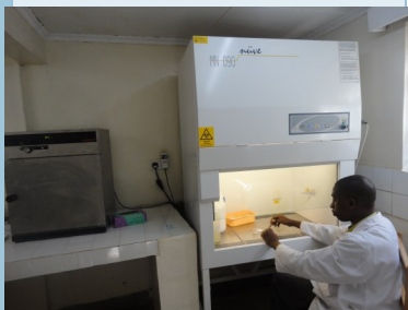
A class 2 Biosafety Cabinet for Microbiology
